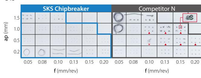
Cutting Conditions : Vc = 100 m/min, Wet, DCGT11T302 Type
