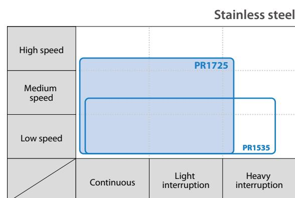
**PR1725: For general purpose high-speed machining**
