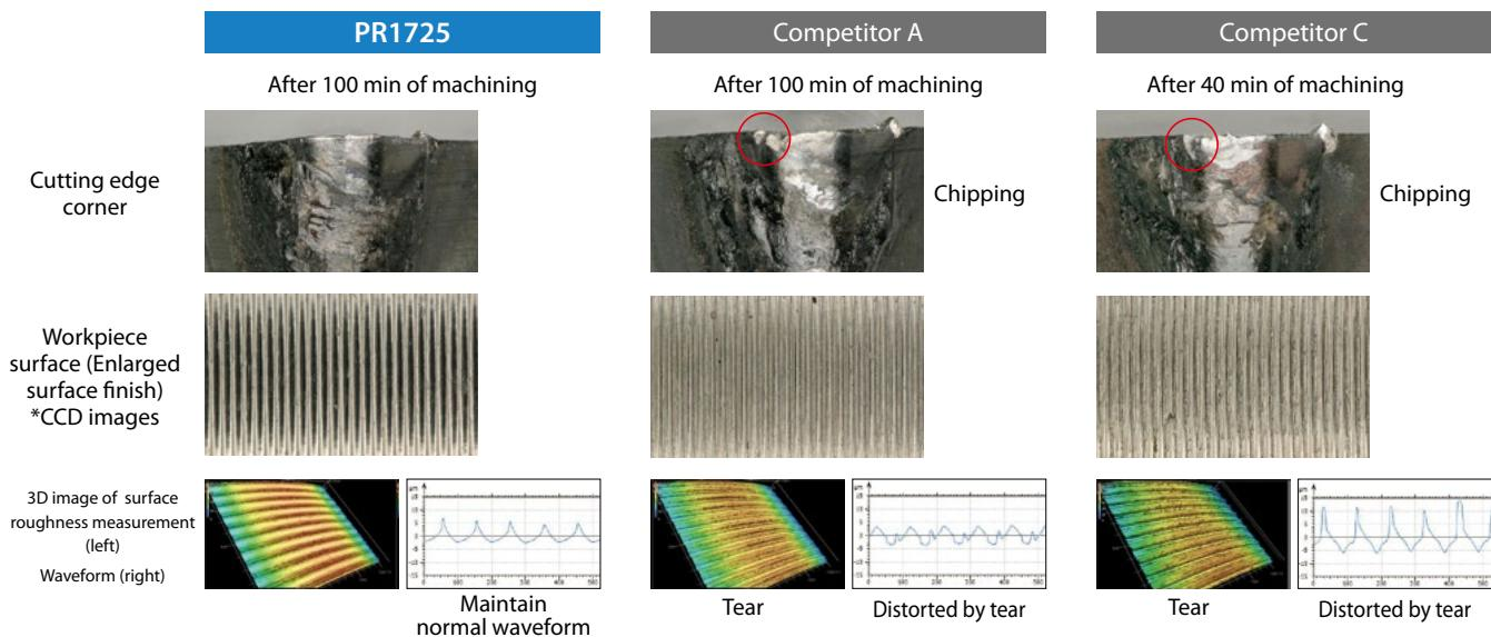
**PR1725 shows less damage on the cutting edge and maintains stable tool mark on the workpiece surface**
