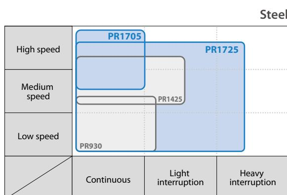
**PR1725: 1st recommendation for steel machining**
