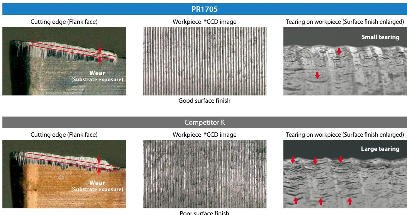
PR1705 showed little adhesion to the cutting edge and good surface finish on the workpiece without tearing
