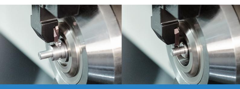
Low cutting force with a large rake angle for high precision grooving
