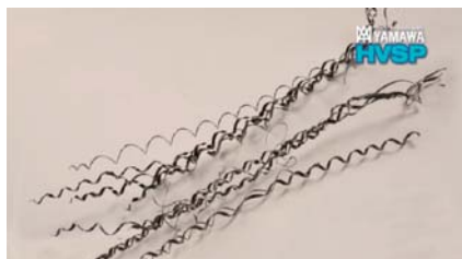
Ejected chips by large size taps
