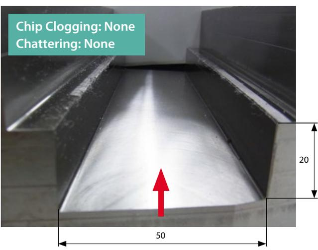
Cutting conditions:  $V_c = 40$  m/min,  $ap \times ae = 20 \times 50$  mm (Slotting),  $f_z = 0.08$  mm/t  $\phi 50$  (5 Flutes), wet (external and internal coolant), workpiece: Ti6Al4V Machine: BT50
