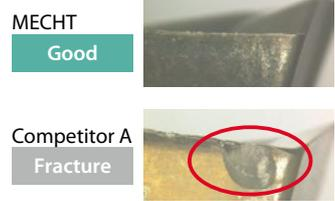
Cutting conditions:  $V_c = 40$  m/min,  $ap \times ae = 43 \times 20$  mm,  $f_z = 0.12$  mm/t,  $\phi 50$  (5 Flutes), wet (external and internal coolant), workpiece: Ti6Al4V Machine: BT50
