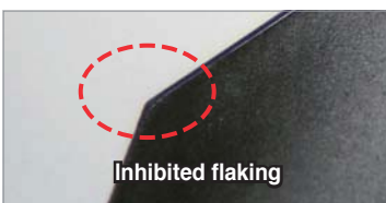
Less wear and flaking on the rake surface
