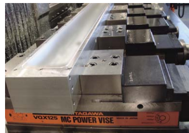
▲長尺物の精密機器部品を加工 ▲Long-size precision equipment parts are machined.
