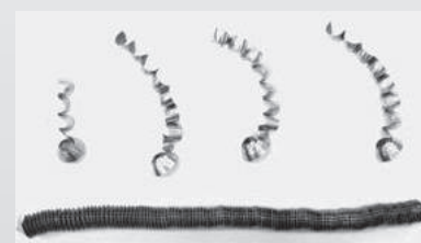
Chips by SM chipbreaker (SUS304)
